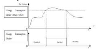
Figure 7-39 Energy consumption brake
