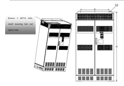
Figure 11-7 Installation of Upper Mounting Hole
