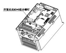
Figure 6 IO expansion card installation diagram
