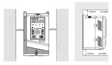
Figure 2-2 Inverter Installation Direction and Space
