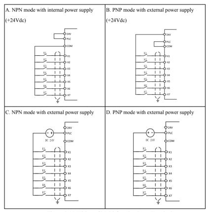
Figure 3-17 Wiring of Multi-function Input Terminals
