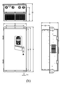
Figure 2-8 Installation Dimensions for Flush Mounting
