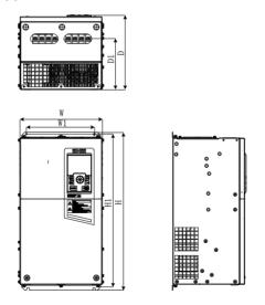
(c) Overall Dimensions of 22 kW – 75 kW Inverters
