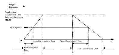
Figure 7-33 Acceleration/Deceleration Time
