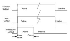
Figure 7-14 Numeric Output Terminal Level and Monopulse Output
