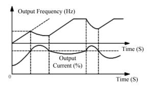
Figure 7-25 Current Limit Action Procedure
