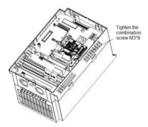
Figure 3 Installation of Profibus-DP expansion card
