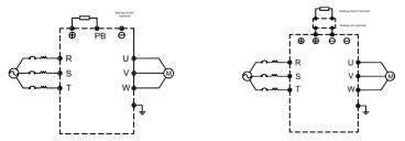
Figure 3-4 Standard Wiring of Main Circuit
