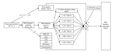
Figure 1-2 Main Frequency Source A Setting
