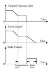
Figure 7-18 Start Process of DC Brake
