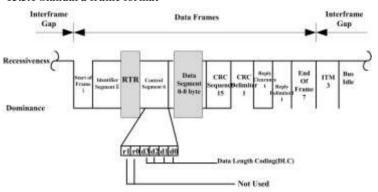
**A frame header** is used to indicate the beginning of a data frame or remote frame, as a definite dominant bit.
