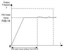
Figure 7-29 PID Initial Value Output
