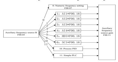
Figure 1-3 Auxiliary Frequency Source B Setting
