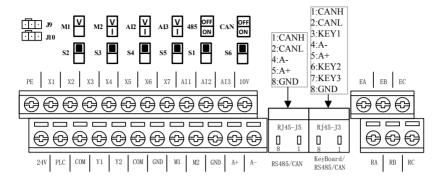
Figure 3-12 Control Circuit Terminal Block
