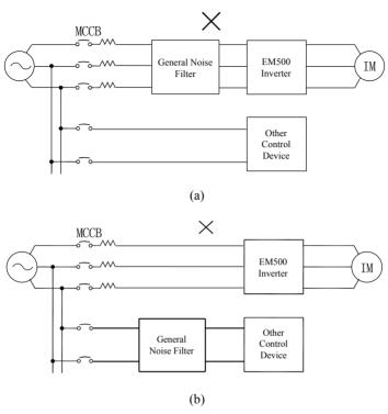
Figure 3-7 Incorrect Installation of Noise Filter
