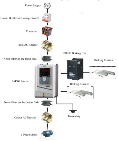
Figure 3-1 Connection of EM500 Inverter and Peripherals
