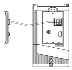
Figure 3-25 Wiring of Keypad Extension Line
