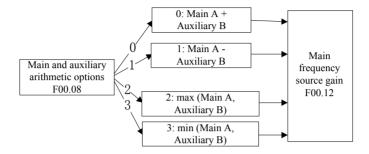
Figure 1-4 Main and Auxiliary Arithmetic Setting
