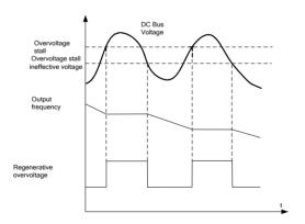
Figure 7-24 Overvoltage Stall Protection
