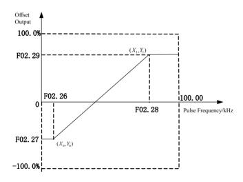
Figure 7-10 High-Speed Pulse Input Offset Curve
