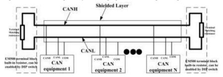
Figure 13-1 CAN bus topology diagram
