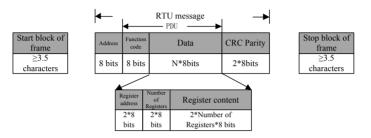
Figure 12-1 RTU Message Frame
