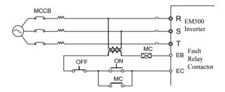
Figure 3-5 Connecting to Input Circuit Breaker
