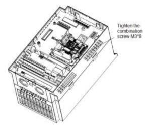
Figure 5 Installation of DeviceNet Expansion Card
