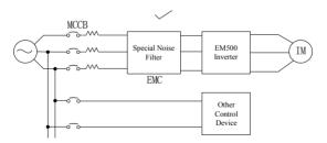
Figure 3–6 Correct Installation of Noise Filter
