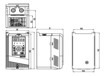
(b) Overall Dimensions of 0.75 kW – 18 kW Inverters
