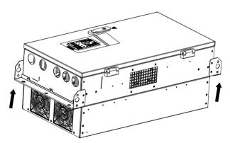
Figure 2-6 Assemble Top and Bottom Mounting Holes
