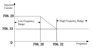
Figure 7-23 High Frequency Injection
