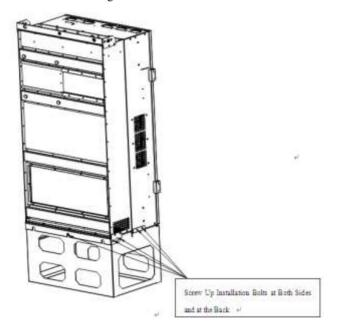
Figure 11–3 Base Installation
