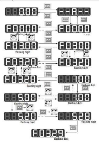
Figure 4-3 Operation Procedure from Power-on to Setting F03.28=5.28
