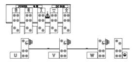
g) Main Circuit Terminal Block of Models 450 - 560 kW Figure 3–2 Main Circuit Terminal Block
