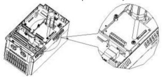
Figure 1 Installation of IO Expansion Card
