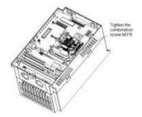
Figure 4 CANopen Expansion Card Installation
